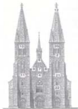
Figure 11. Measuring points in the façade (ITAM, 2002)
