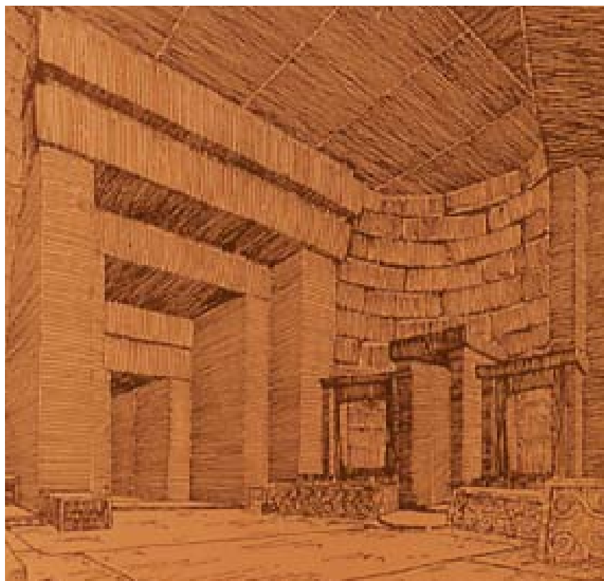
Fig. 10 - Restoration of an interior of the prehistoric megalithic Temple of Mnajdra, the vault of which is completed with lithic slabs (C. Ceschi, 1939).
