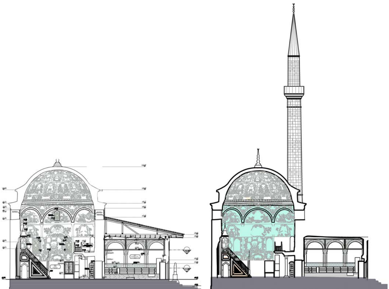
Figure 2: Cross section of Ethem Bey Mosque [11].
