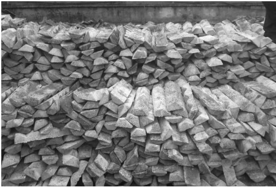
FIGURE 1. Ingots of pig iron smelted near the mine were easily handled and transported to the foundry, where it could be cast or wrought. Source: http://equatorline.indonetwork.co.id/2279287/pig-iron-iron-scrap-roll-coil.htm , accessed November 2012.
