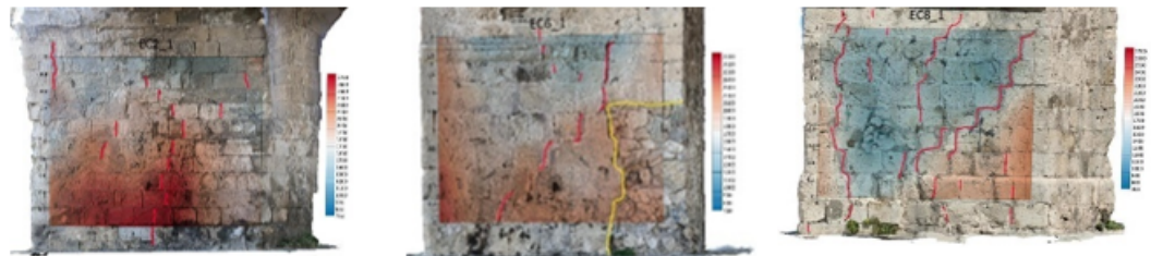
Figure 2: Application of direct sonic test results showing the wave velocity in m/s overlaid on the west elevation of three damaged piers of Eastern Neoria, along with their corresponding crack maps.
