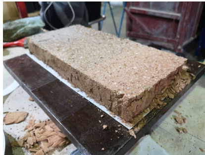
Handmade solid fired-clay brick specimen tested in compression with a PTFE bearing layer to minimise confinement
