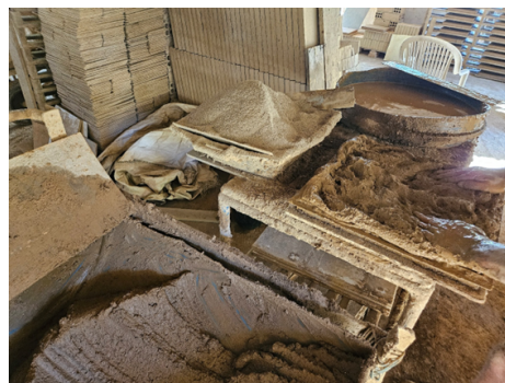
Handmade moulded brick manufacture
