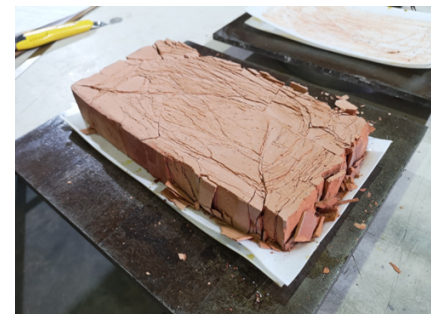
Extruded solid fired-clay brick specimen tested in compression with a PTFE bearing layer to minimise confinement
