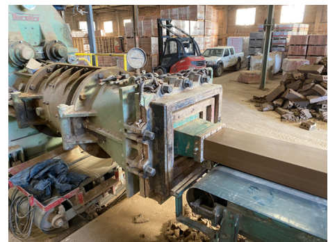
Brick extrusion process, prior to cutting
