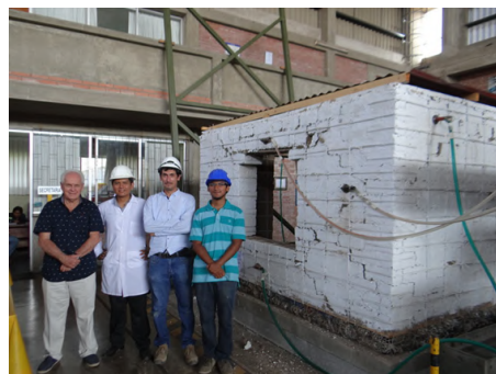
Julio Vargas and collaborators after a shaking table test of an isolated and reinforced adobe dwelling
