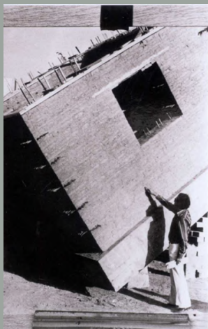
Julio Vargas in 1975 testing a reinforced adobe dwelling on the tilt-up table
