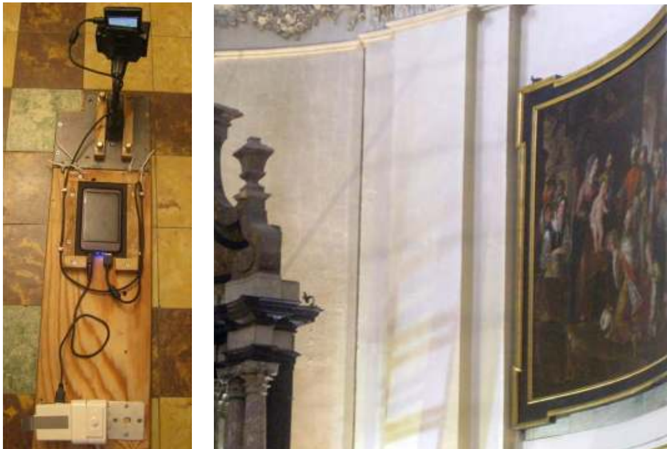
Figure 30. Displacement monitoring using a smartphone: left, equipment; right, smartphone position on the altar's cornice in front of the canvas.
