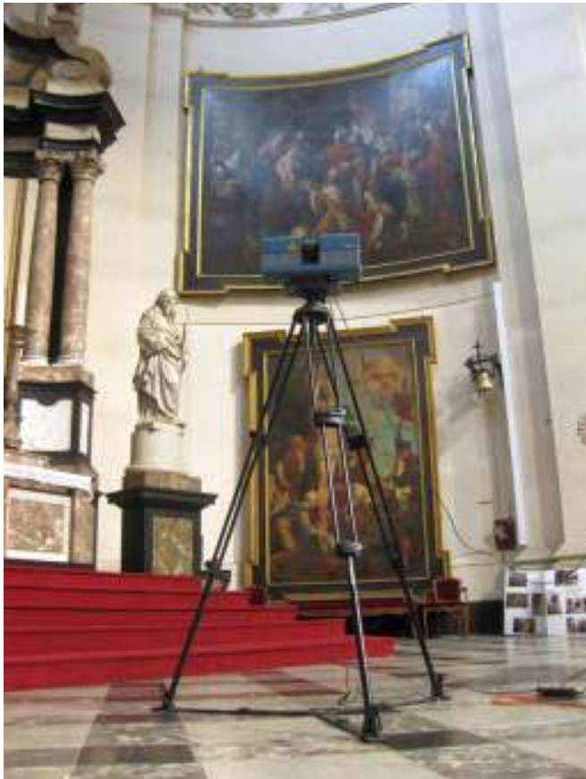
Figure 11. St. Aubain Cathedral in Namur, Belgium. Left, scanning of the curvilinear painting “Adoration of the Magi”. Right, scan preview with visible two holes in the upper part of the painting.
