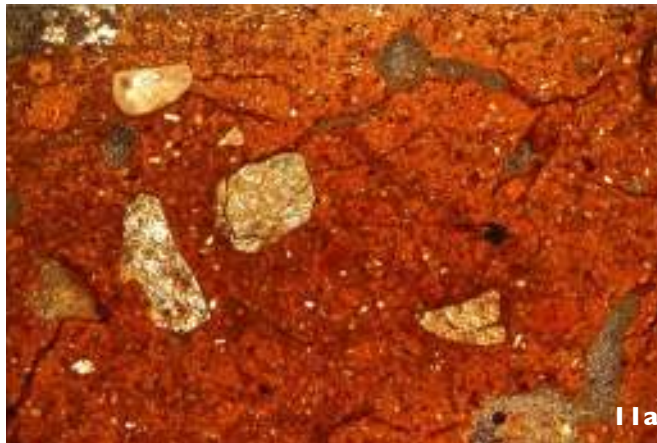
Figures 11a. Lime crumbs in old brick of the minaret, 11b. lime and quartz crumbs in old mortar of the minaret.
