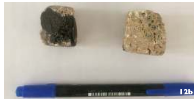
Figures 11a. Lime crumbs in old brick of the minaret, 11b. lime and quartz crumbs in old mortar of the minaret.
