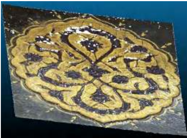
Figure 16. Model of the cover ornament based on the laser triangulation scanning.
