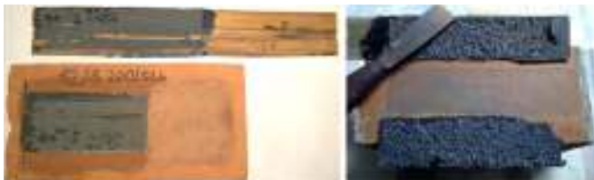
Figures 30. Reversibility of polyurethane PS flexible adhesive – easy removable with a spatula [19].
