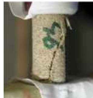
Figure 28. Sequence of the strength tests using a micro-core: left, FS; middle, UCS; right, ITS.
