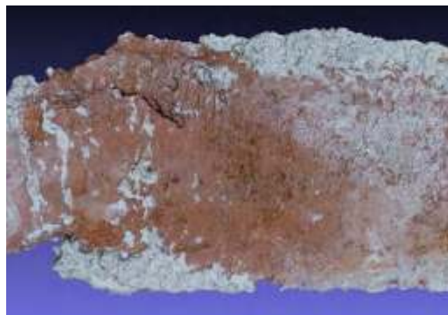
Figure 17. Hand-held camera photogrammetric model of a brick surface (left). Crack points coordinates shown in Cloud Compare (right).
