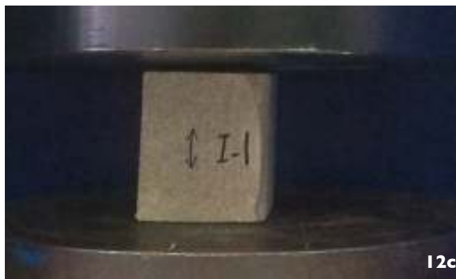
Figures 12. Materials samples in the foundation: 12a. adobe, 12b. mortar, 12c. stone, 12d. stress-strain diagram of dry adobe.
