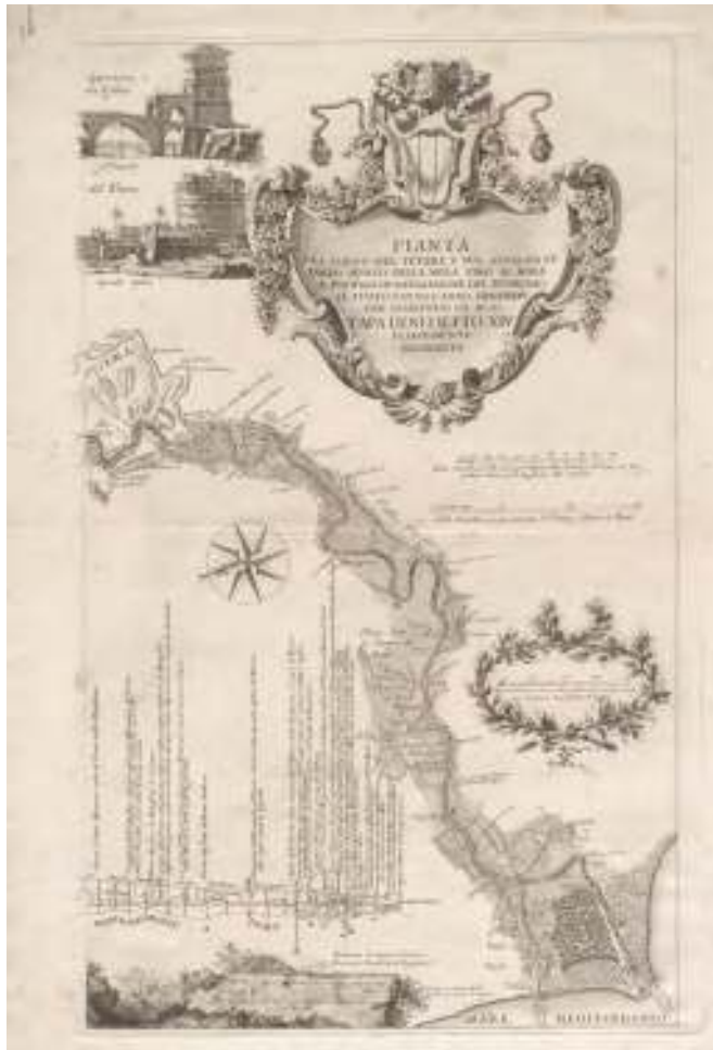
Map of the Tiber River between Rome and its mouth in the Tyrrhenian Sea. The survey, conducted by Bolognese engineers Gambarini and Chiesa in 1744, shows the river's course and the depth of its bed.
