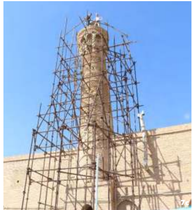
Figures 7. Vibration test: 7a. the locations of sensors (accelerometers), 7b. sensor at mid-height of the minaret, 7c. generating vibration in the minaret by hands, 7d. generating harmonic ground vibration using heavy rollers.
