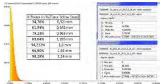
Figure 12. St. Aubain Cathedral in Namur, Belgium. Left, histogram of the point distance differences between two scans. Right, statistics of distance computation for two scans compared with the reference one.
