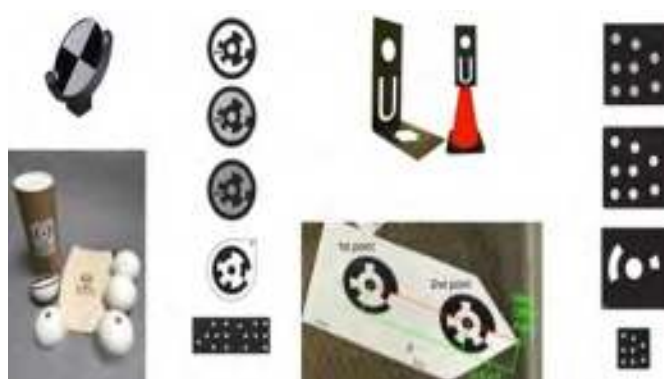
Figure 1. Coded and non-coded targets used in photogrammetry and laser scanning.
