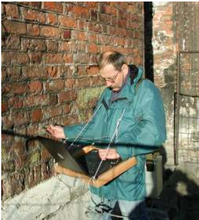
Figure 23. In-situ measurements using edge probes: left, St. John's church in Gdańsk (Poland); right, Santa Maria del Fiore in Florence (Italy).
