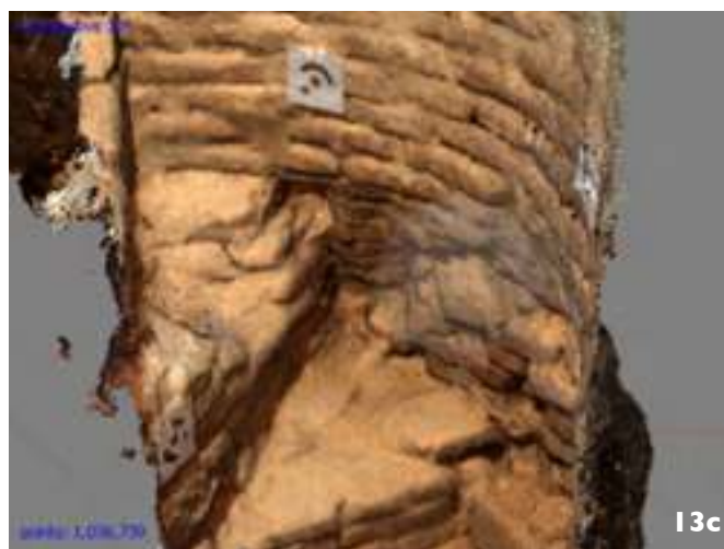
Figures 13. Close range photogrammetry of the minaret, cloud point samples: 13a. outer side, 13b. close-up outer side, 13c. and 13d. inner side.
