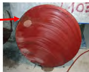
b) Testing the spread of the resin (red color) inside the flat jack
