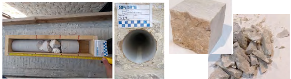
Extraction of wall structure and laboratory testing samples
