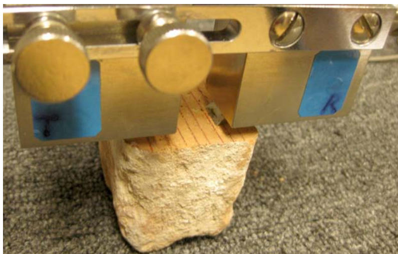
Figure 5: Surface Rayleigh wave VR propagating in X-direction measured with edge probes (left) by signal correlation method.
