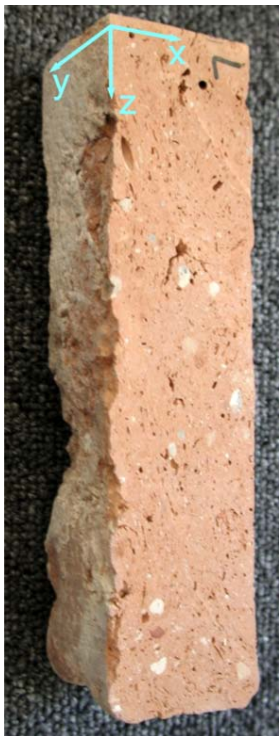
Figure 4: Sample of the brick from Puerta de Burgos with sample coordinate system (left) and drilled micro-core specimens (right).
