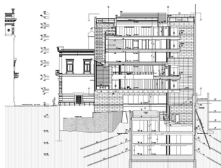
Figs. 14 & 15. Cross sections T1 and T4 of the National Bank of Greece Administration Building with the antiquities preserved in the ground floor – basement. The underground floors below the antiquities are also shown.
