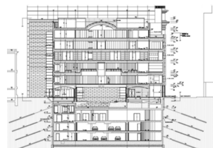
Figs. 14 & 15. Cross sections T1 and T4 of the National Bank of Greece Administration Building with the antiquities preserved in the ground floor – basement. The underground floors below the antiquities are also shown.
