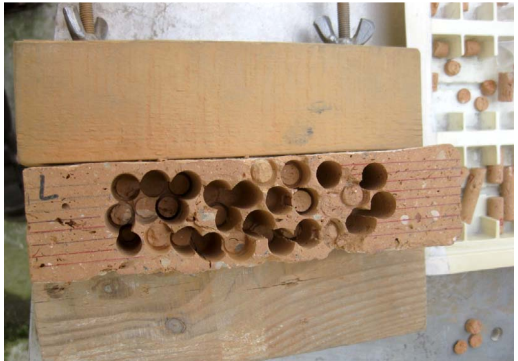
Figure 4: Sample of the brick from Puerta de Burgos with sample coordinate system (left) and drilled micro-core specimens (right).
