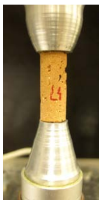
Figure 7: Recording of longitudinal VP wave in a brick specimen from Puerta de Burgos.
